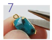
Set it in a square setting and hold the resin stone with holding pins.
