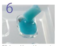
Fill the mold up with turquoise resin and cure it in a minute. After cooling down, take it out.
