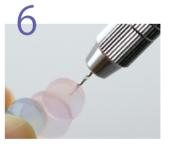
Make a hole on the end dots with a pin vise.
