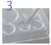
Drop different colored resin next to the first one. Repeat that until the mold be filled up with resin. Cure in 1 minute under UV-LED light.
