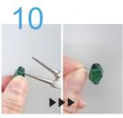
Push the stick from both sides using a round nose pliers. Once the stick moves and comes out, pull it out by hands.
