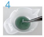
Hold an 8mm-cut stick with tweezers and dip both tips of the stick a bit into the colored resin.
