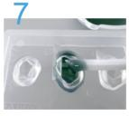
Scoop the resin and place it into the mold with a mixing stick. Be careful not to take the fixed stick off by hitting it
